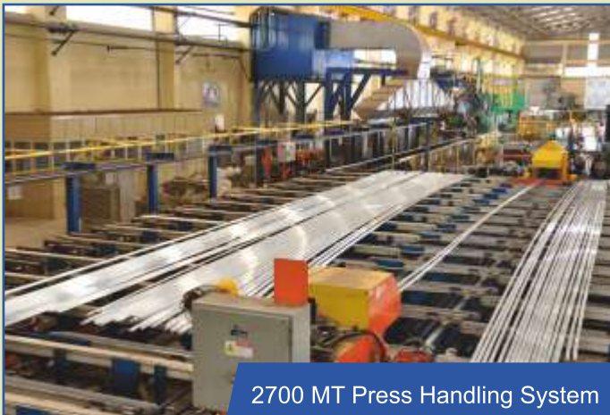
2700 MT Press Handling System
